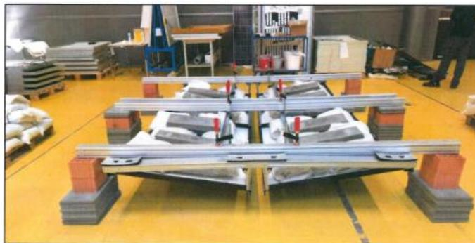
[Bild 3: Windlast-Abhebeversuch]
